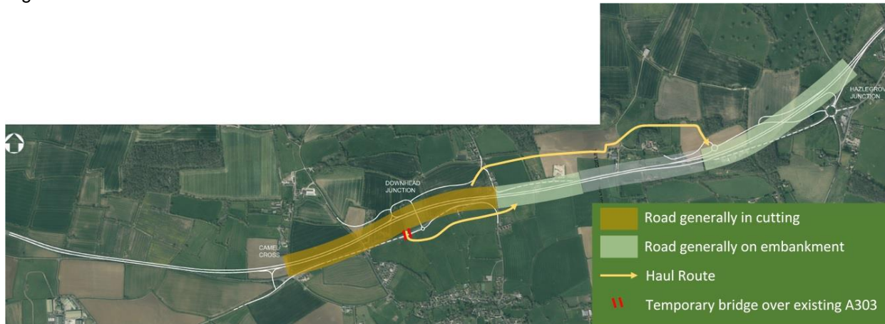
Figure 2.19: Main earthworks areas of the scheme
